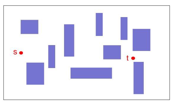
Robot always knows its current position and the position of t. Does not know in advance the position/extent of the obstacles. Tactile robot: Can touch/sense the obstacles.
