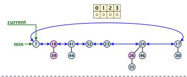
During the consolidation we traverse the root list. Whenever we discover two trees that have the same degree we merge these trees. In order to efficiently check whether two trees have the same degree, we use an array that contains for every degree value d a pointer to a tree left of the current pointer whose root has degree d (if such a tree exist).
