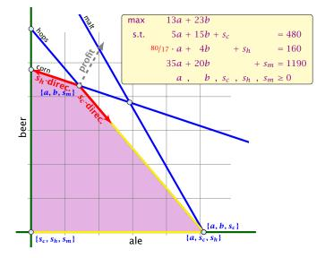
If a basis variable is 0 in the basic feasible solution then we may not make progress during an iteration of simplex.
