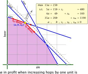
The change in profit when increasing hops by one unit is =  $\underbrace{c_B^T A_B^{-1}}_{\gamma^*} e_h$ . Of course, the previous argument about the increase in the primal objective only holds for the non-degenerate case.
