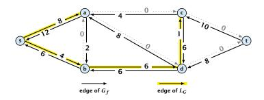
In the following we assume that the residual graph  $\mathcal{G}_f$  does not contain zero capacity edges.
