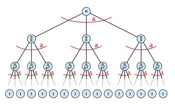
The running time of a recursive algorithm can be visualized by a recursion tree:
