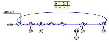
During the consolidation we traverse the root list. Whenever we discover two trees that have the same degree we merge these trees. In order to efficiently check whether two trees have the same degree, we use an array that contains for every degree value d a pointer to a tree left of the current pointer whose root has degree d (if such a tree exist).
