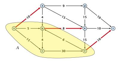
The capacity of the cut is  $cap(A, V \setminus A) = 28$ .
