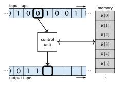
Note that in the picture on the right the tapes are one-directional, and that a READ- or WRITE-operation always advances its tape.
