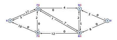
Note that the lemma is almost trivial. A node v having excess flow means that the current preflow ships something to v. The residual graph allows to  $\mathit{undo}$  flow. Therefore, there must exist a path that can undo the shipment and move it back to s. However, a formal proof is required.
