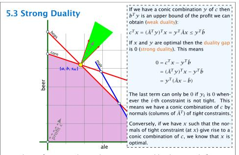
The profit vector c lies in the cone generated by the normals for the hops and the corn constraint (the tight constraints).
